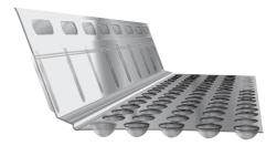
ECP Water Channel – The ECP Water channel is an interior basement floor drainage system for new construction and retrofitting. Engineered to sit on top of the footing to create a pathway for water to flow from the wall and cold joint, across the footing and into the drain system. This unique design provides added strength to the channel to prevent collapsing and warping along the wall and creates a thermal break between the footing and slab.
