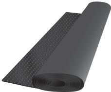
Dimple Drainage Board – Sheet Drains for single side drainage applications are prefabricated products that consist of a solid, formed, three dimensional core covered with a geo-textile filter fabric bonded to the dimple side of the core.
