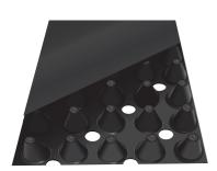
ECP Strip Drain – ECP Strip Drains are prefabricated drains that consist of a high-profile, perforated, three-dimensional core (6" high x 1" wide x 150' long) that is fully wrapped with a filter fabric.
