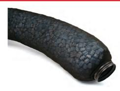
EZ Flow Gravel Free French Drain System – EZflow is a gravel-free alternative to a traditional French Drain system. Each EZflow section contains a 10 foot-long plastic corrugated pipe surrounded by EZflow Poly Rock aggregate structurally engineered to have an increased void space. Pipe and aggregate are enclosed in a strong and durable mesh material to prevent clogging.
